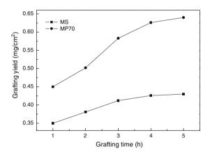
Fig. 4. Effect of surface morphology on the grafting yield of PAA. MS: nonporous surface; MP70: porous surface.
