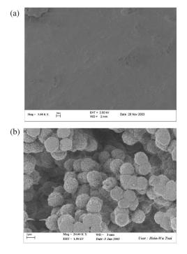
Fig. 1. Dense and porous PVDF membrane surfaces for grafting PAA. (a) MS; (b) MP70.
