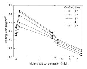
Fig. 3. Effect of Mohr's salt concentration  $(1.5 \times 10^{-5} - 7.5 \times 10^{-3} \text{ M})$  on the grafting yield of PAA. Substrate: membrane 'MP70'; Plasma power: 100 W; Plasma irradiation time: 60 s.
