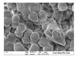
Fig. 5. SEM photomicrograph of membrane MP70 after being grafted with  $0.64 \text{ mg/cm}^2$  of PAA.
