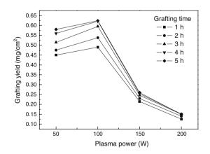
Fig. 7. Effect of plasma power (50–200 W) on the grafting yield of PAA on membrane 'MP70'. The concentration of the Mohr's salt was  $1.5 \times 10^{-4}$  M, and the plasma treatment time was 60 s.
