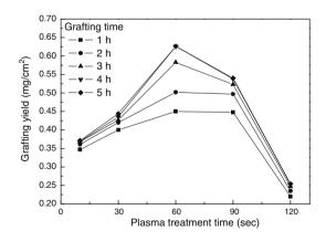
Fig. 6. Effect of plasma treatment time (10–120 s) on the grafting yield of PAA on membrane 'MP70'. The concentration of the Mohr's salt was  $1.5 \times 10^{-4}$  M, and the plasma power was 100 W.
