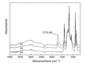
Fig. 2. FTIR-ATR spectra of primitive PVDF membrane and PAA/PVDF composite membranes. (a) Primitive PVDF membrane, MP70; (b) PAA/PVDF composite membrane, grafting yield 0.39 mg/cm<sup>2</sup>; (c) PAA/PVDF composite membrane, grafting yield 0.64 mg/cm<sup>2</sup>.
